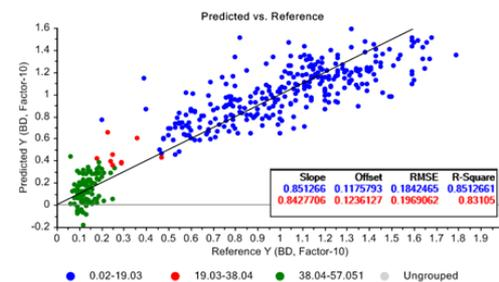
Calibration results for the prediction of Bulk Density (NIR)
