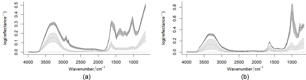
**Figure 3. Mean +/- standard deviation of 10 laboratory ATR measured MIR spectra of fresh soil samples (dark grey) and 10 in-field ATR measured MIR spectra (light grey) from two Swedish soils; a) organic soil, and b) mineral soil.**
