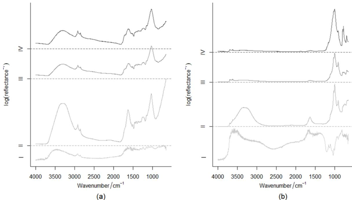
**Figure 4. Laboratory measured MIR spectra from two Scottish soils; a) organic soil, and b) mineral soil. I) are fresh samples measured using diffuse reflectance. II to IV are measured using DATR on II) fresh, III) dried, IV) dried and milled soil samples.**
