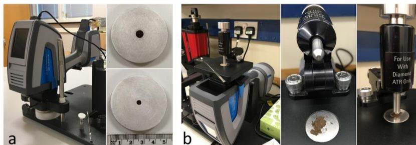
Figure 1. Laboratory setup for a) diffuse reflectance measurements with two powder sampling puck sizes, and b) DART measurements using a small field clip.
