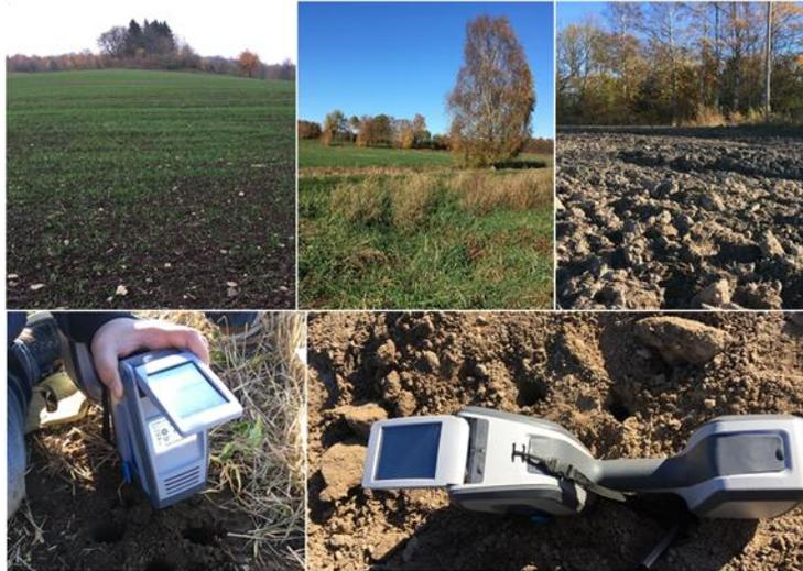
**Figure 2. In-field measurements using ATR pressing the instrument on to the soil for contact. Also visible are some of the holes from the soil samples that were taken for laboratory measurements.**
