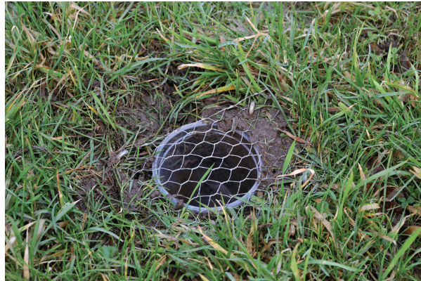
Mesh grid in place on top of collection pot
